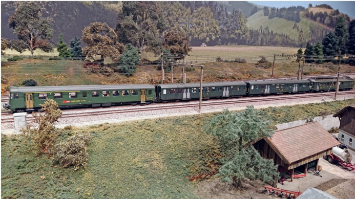
BDe 4/4, 1,18 MW, 59 t, Last: 12 A, 98 t, total 242 Pl., 157 t, V max 110 km/h.
