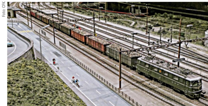
Ae 6/6, 6000 PS/4,3 MW, 120 t, Last: 32 Achsen, 544 t, V/max 100 km/h.
