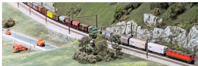
Ae 6/6, 6000 PS/4,3 MW, 120 t, Last: 44 Achsen, 780 t, V max 100 km/h.
